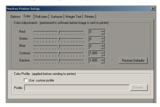
Photographic printers have an on-board linearization process that should be performed immediately prior to printing the testchart. Noritsu minilab owners should perform an emulsion change twice in a row (the second round improves linearization).
